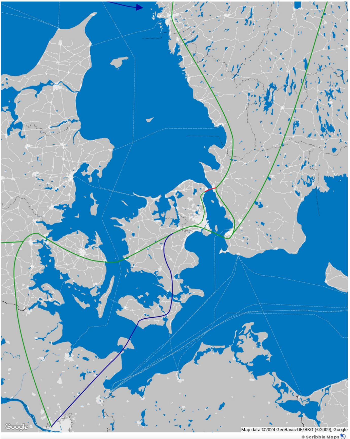
Figure 4 - Map of railways between Germany and Sweden. Green are established lines, blue is the coming Fehmarn Belt line, and the dotted red line is the proposed Helsingør-Helsingborg link. Map by Risk Intelligence.
